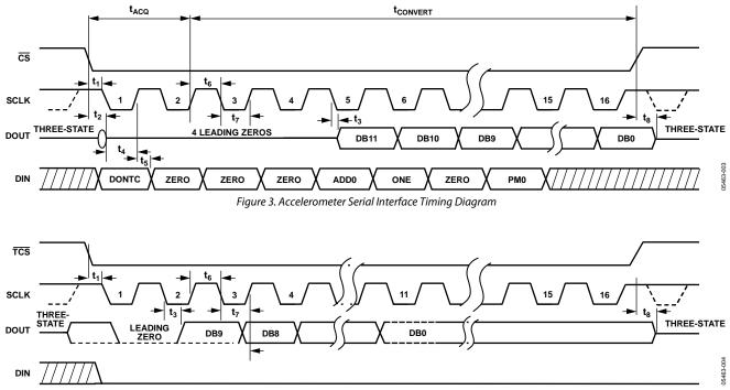
Figure 4. Temperature Serial Interface Timing Diagram
