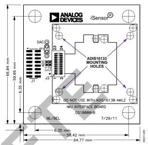
Figure 21. Physical Diagram for the Current ADIS16IMU1/PCBZ
