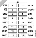
Figure 22. ADIS16IMU1/PCBZ J1 Pin Assignments
