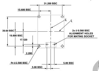
Figure 23. Suggested Mounting Hole Locations, Connector Down
