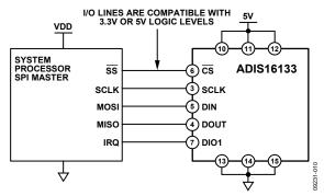
Figure 10. Electrical Connection Diagram
