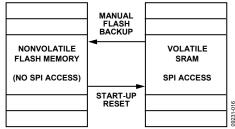
Figure 16. SRAM and Flash Memory Diagram
