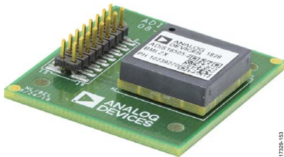
Figure 64. ADIS16507-2 Breakout Board (ADIS16505-2 Shown)
