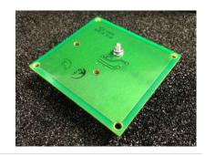
4 Repeat the process with the other two machine screws, then use a torque screw driver to tighten the machine screw torque to 24 inch-ounces.
