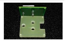
6 Mount the interface board and spacer to the test surface using the machine screws
