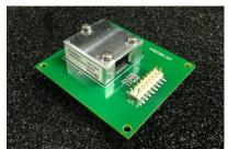
5 Set the interface board (with IMU installed) on top of the spacer
