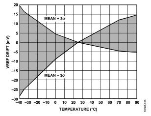
Figure 18. VREF Drift vs. Temperature (3 σ to Either Side of Mean)
