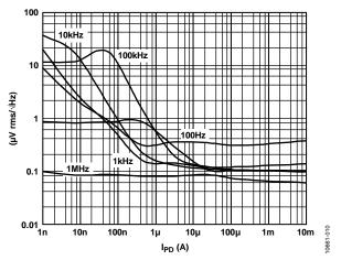
Figure 10. Spot Noise Spectral Density at V<sub>LOG</sub> vs. I<sub>PD</sub>
