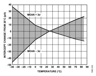
Figure 20. Intercept Drift vs. Temperature (3 σ to Either Side of Mean)
