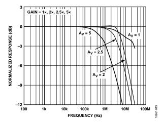
Figure 13. Small Signal Response of Buffer
