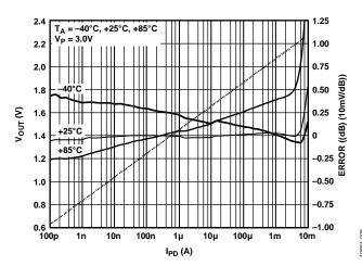
Figure 8. Logarithmic Conformance (Linearity) for a 3 V Single Supply
