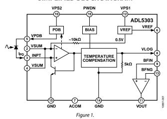
input pin INPT is flanked by the VSUM guard pins that track the voltage at the summing node. Connecting the exposed pad of the device to the VSUM pins provides a continuous guard to minimize leakage into the INPT pin.
