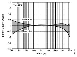
Figure 15. Logarithmic Conformance Error Distribution (3 σ to Either Side of Mean)
