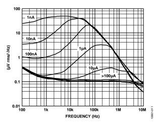
Figure 11. Spot Noise Spectral Density at V<sub>LOG</sub> vs. Frequency
