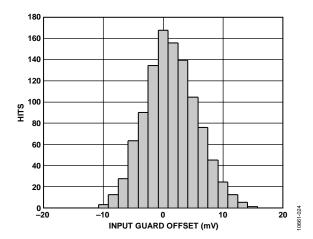
Figure 24. Distribution of Input Guard Offset Voltage V<sub>OFS</sub> (V<sub>INPT</sub> – V<sub>SUM</sub>)
