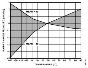
Figure 19. Slope Drift vs. Temperature (3 σ to Either Side of Mean)
