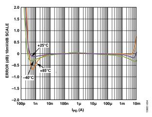
Figure 4. Logarithmic Conformance (Linearity) for V<sub>LOG</sub>
