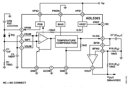
Figure 29. Using the Adaptive Biasing
