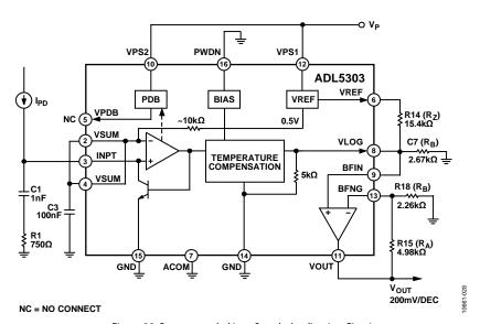
Figure 28. Recommended Low Supply Application Circuit
