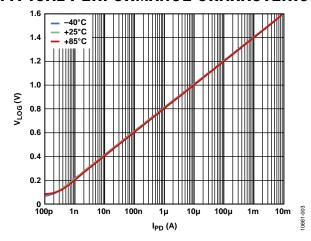
Figure 3.  $V_{LOG}$  vs.  $I_{PD}$
