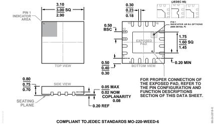
Figure 34. 16-Lead Lead Frame Chip Scale Package [LFCSP] 3 mm × 3 mm Body and 0.75 mm Package Height (CP-16-22) Dimensions shown in millimeters
