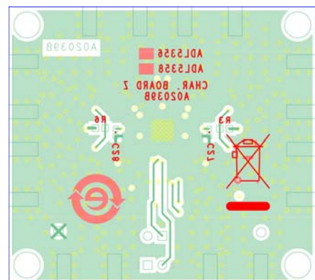
Figure 56. Evaluation Board Bottom Layer
