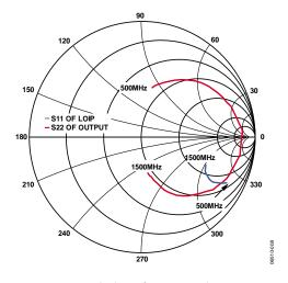
Figure 8. Smith Chart of LOIP S11 and VOUT S22 ( $f_{LO}$  from 500 MHz to 1500 MHz)
