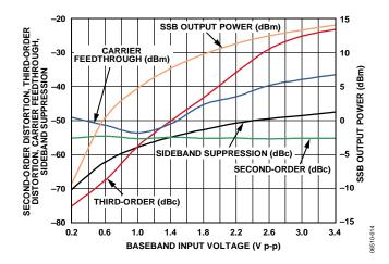
Figure 14. Second- and Third-Order Distortion, Carrier Feedthrough, Sideband Suppression, and SSB  $P_{OUT}$  vs. Baseband Differential Input Level ( $f_{LO} = 900 \text{ MHz}$ )
