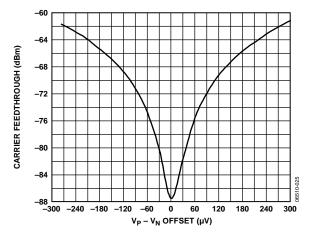
Figure 24. Typical Carrier Feedthrough vs. DC Offset Voltage
