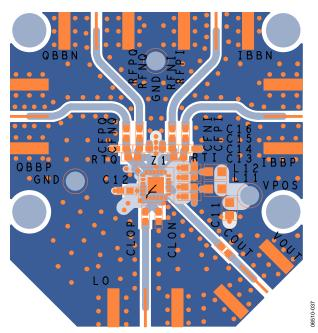
Figure 35. Evaluation Board Layout, Top Layer
