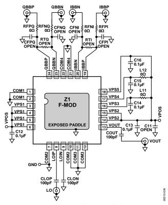
Figure 34. ADL5371 Evaluation Board Schematic
