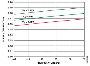
Figure 20. Power Supply Current vs. Temperature
