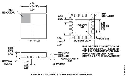
Figure 38. 24-Lead Lead Frame Chip Scale Package [LFCSP] 4 mm × 4 mm Body and 0.75 mm Package Height (CP-24-14) Dimensions shown in millimeters
