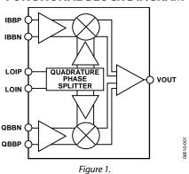
The ADL5371 accepts two differential baseband inputs and a single-ended local oscillator (LO) and generates a single-ended output.
