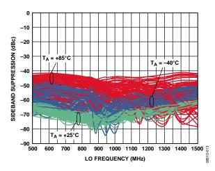
Figure 13. Sideband Suppression vs. f<sub>LO</sub> and Temperature After Nulling at 25°C (Multiple Devices Shown)
