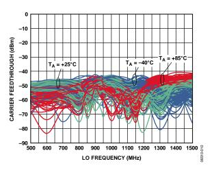
Figure 10. Carrier Feedthrough vs. f<sub>LO</sub> and Temperature (Multiple Devices Shown)
