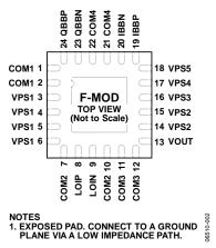
Figure 2. Pin Configuration
