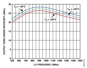
Figure 17. OIP3 vs. Frequency and Temperature
