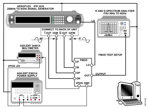
Figure 36. Characterization Bench Setup
