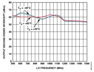
Figure 18. OIP2 vs. Frequency and Temperature
