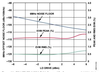
Figure 33. GSM/EDGE (8 PSK) EVM, Spectral Performance, and 6 MHz Noise Floor vs. LO Power at 940 MHz; Output Power = 5 dBm
