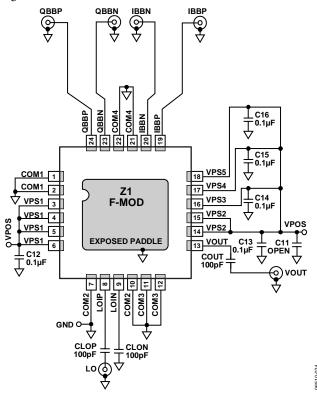
Figure 23. Basic Connections for the ADL5371
