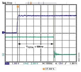
Figure 18. OrFET Turn-On Time (Default Polarity)
