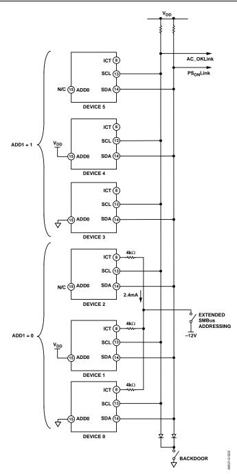
Figure 38. Extended SMBus Addressing and Backdoor Access
