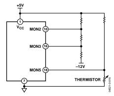
Figure 22. Example of MON Pin Configuration
