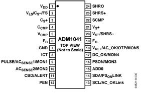
Figure 7. Pin Configuration
