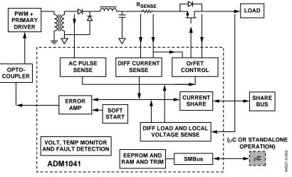
Figure 2. Application Block Diagram
