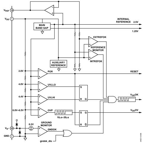
Figure 8. Block Diagram of Power Management Section
