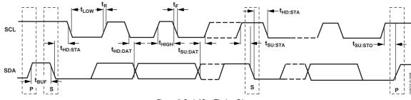
Figure 5. Serial Bus Timing Diagram
