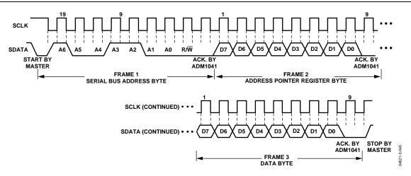
Figure 25. Writing a Register Address to the Address Pointer Register, then Writing Data to the Selected Register
