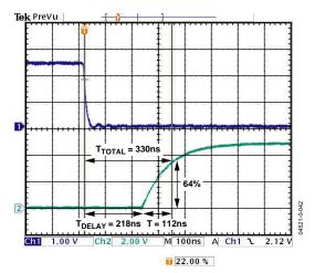
Figure 17. OrFET Turn-Off Time (Default Polarity)
