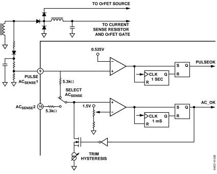
Figure 16. Pulse In and AC Sense Circuit
