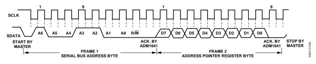
Figure 26. Writing to the Address Pointer Register Only
