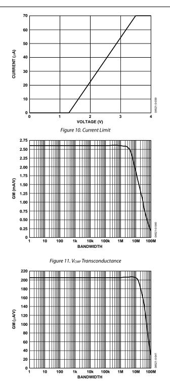
Figure 12. C<sub>CMP</sub> and S<sub>CMP</sub> Transconductance
