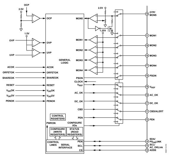
Figure 23. Block Diagram of Protection and General Logic
