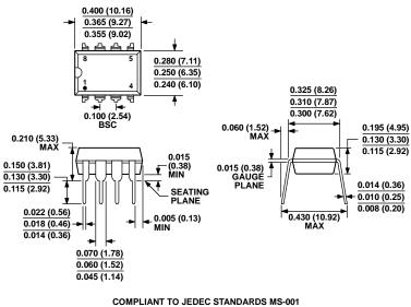
CONTROLLING DIMENSIONS ARE IN INCHES; MILLIMETER DIMENSIONS (IN PARENTHESES) ARE ROUNDED-OFF INCH EQUIVALENTS FOR REFERENCE ONLY AND ARE NOT APPROPRIATE FOR USE IN DESIGN. CORNER LEADS MAY BE CONFIGURED AS WHOLE OR HALF LEADS.
