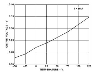
TPC 4. Receiver Output Low Voltage vs. Temperature
