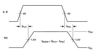
Figure 3. Receiver Propagation Delay
