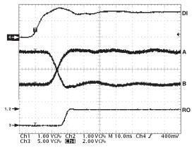
TPC 15. Driver/Receiver Propagation Delays Low to High
