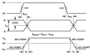
Figure 1. Driver Propagation Delay, Rise/Fall Timing
