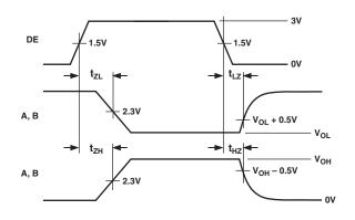
Figure 2. Driver Enable/Disable Timing
