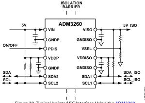
Figure 20. Typical Isolated I<sup>2</sup>C Interface Using the ADM3260
