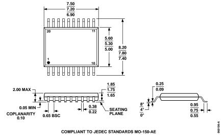
Figure 28. 20-Lead Shrink Small Outline Package [SSOP] (RS-20) Dimensions shown in millimeters
