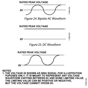
Figure 26. Unipolar AC Waveform
