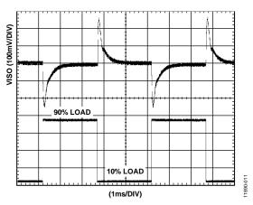
Figure 11. Typical VISO Transient Load Response, 5 V Input, 3.3 V Output, 10% to 90% Load Step
