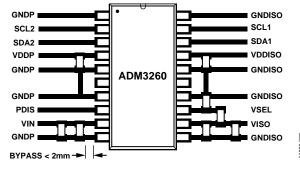
Figure 23. Recommended PCB Layout
