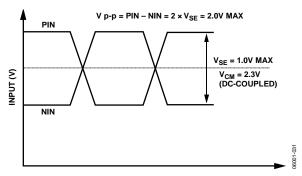
Figure 42. Maximum Allowed DC-Coupled Input Levels
