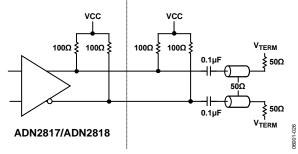
Figure 37. Typical ADN2817/ADN2818 Applications Circuit
