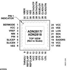
NOTES 1. THE EXPOSED PADDLE ON THE BOTTOM OF THE PACKAGE MUST BE CONNECTED TO VEE.
