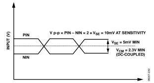
Figure 41. Minimum Allowed DC-Coupled Input Levels
