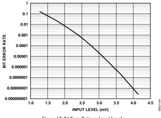
Figure 17. Bit Error Rate vs. Input Level
