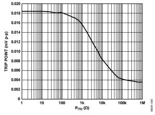
Figure 6. LOS Comparator Trip Point Programming
