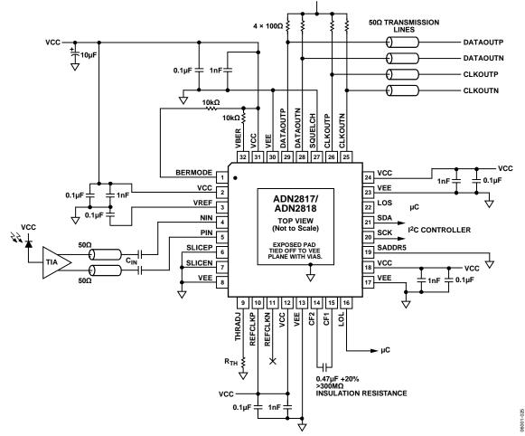
Figure 36. Typical ADN2817/ADN2818 Applications Circuit
