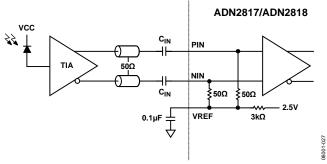
Figure 38. ADN2817/ADN2818 AC-Coupled Input Configuration
