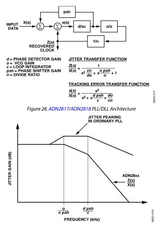
Figure 29. ADN2817/ADN2818 Jitter Response vs. Conventional PLL
