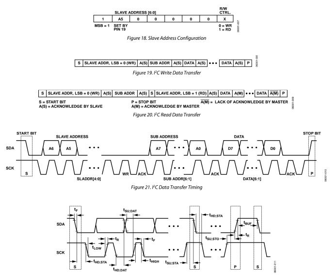
Figure 22. I<sup>2</sup>C Port Timing Diagram
