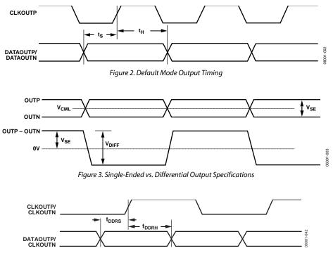
Figure 4. Double Data Rate Mode Output Timing
