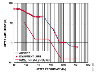
Figure 11. Jitter Tolerance, OC-3
