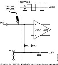
Figure 24. Single-Ended Sensitivity Measurement
