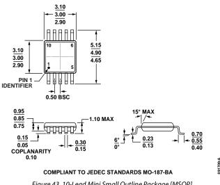
Figure 43. 10-Lead Mini Small Outline Package [MSOP] (RM-10) Dimensions shown in millimeters
