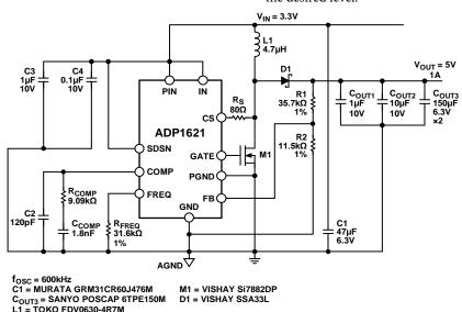
Figure 33. Typical Boost Converter Application Circuit
