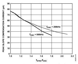
Figure 19. Slope-Compensation Current vs. fsync/fosc
