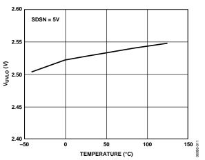
Figure 12. V<sub>UVLO</sub> Threshold vs. Temperature
