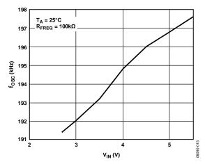
Figure 16. Oscillator Frequency vs. V<sub>IN</sub>
