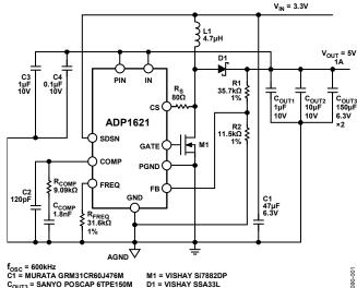
f<sub>osc</sub> = 600kHz C1 = MURATA GRM31CR60J476M M1 = VISHAY S17882DP C<sub>OUT3</sub> = SANYO POSCAP 6TPE150M D1 = VISHAY SSA33L L1 = TOKO FDV0630-4R7M Figure 1. High Efficiency Output Boost Converter in Lossless Mode, 3.3 V Input, 5 V Output (Bootstrapped)
