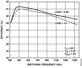
Figure 8. Efficiency vs. Switching Frequency
