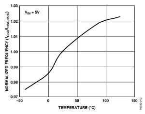
Figure 13. Frequency vs. Temperature
