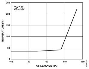
Figure 17. Temperature vs. CS Leakage
