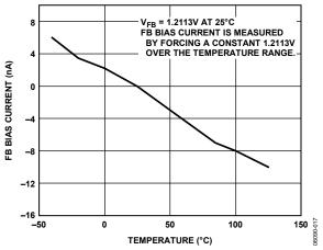
Figure 18. FB Bias Current vs. Temperature
