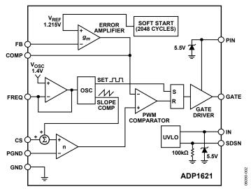
Figure 3. ADP1621 Simplified Block Diagram
