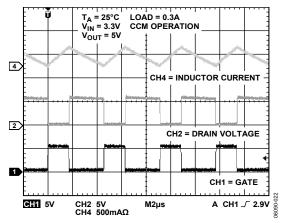
Figure 23. CCM Switching Waveform
