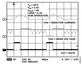
Figure 22. DCM Switching Waveform
