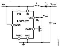
Figure 28. CS Pin Connection for V<sub>SW</sub> < 30 V, Lossless Mode (No Current-Sense Resistor Needed)
