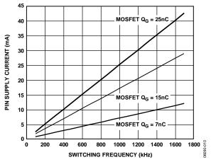
Figure 11. PIN Supply Current vs. Switching Frequency
