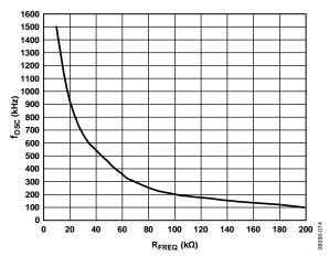
Figure 15. Oscillator Frequency vs. Resistance
