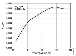
Figure 21. FB Voltage vs. Temperature
