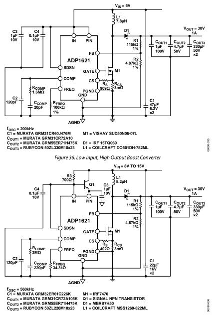
Figure 37. High Input Voltage and High Output Voltage Converter
