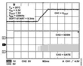
Figure 24. Soft Start Waveform
