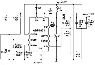
$\begin{aligned} & f_{OSC} = 600 \text{kHz} \\ & \text{C1 = MURATA GRM31CR60J476M} \\ & \text{C}_{OUT2} = \text{RUBYCON 25ZL330M8x16} \\ & \text{L1 = COILCRAFT MSS1260-103ML} \end{aligned} \qquad \begin{aligned} & \text{M1 = IRF7470} \\ & \text{D1 = VISHAY SSC53L} \\ & \text{D2 = SIGNAL DIODE} \end{aligned}$
