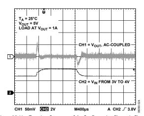
Figure 25. Line Transient Response of the Configuration Shown in Figure 1 with a 1 A Load
