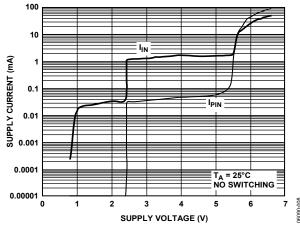
Figure 9. Supply Current vs. Supply Voltage
