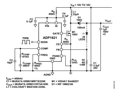
Figure 41. 20-Series LED Driver with PWM at SDSN
