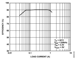
Figure 5. Efficiency vs. Load Current
