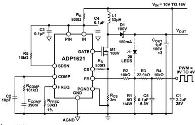
f<sub>OSC</sub> = 400kHz C1 = MURATA GRM31MR71E225K M1 = VISHAY Si4482DY C<sub>OUT</sub> = MURATA GRM31CR72A105K D1 = IRF 10MQ100 L1 = COILCRAFT MSS1038-333NL
