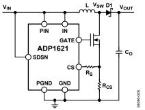
Figure 29. CS Pin Connection for V<sub>SW</sub> > 30 V, Resistor Sense Mode with a Current-Sense Resistor, R<sub>CS</sub>
