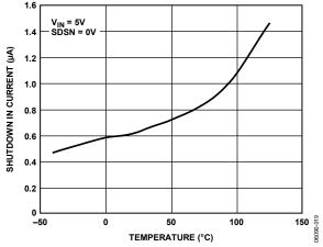
Figure 20. Shutdown IN Current vs. Temperature
