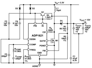
f<sub>OSC</sub> = 600kHz C1 = MURATA GRM31CR60J476M M1 = IRF7470 C<sub>OUT2</sub> = RUBYCON 25ZL330M8x16 D1 = VISHAY SSC53L L1 = COILCRAFT MSS1260-103ML D2, D3 = SIGNAL DIODE Q1 = SIGNAL NPN TRANSISTOR
