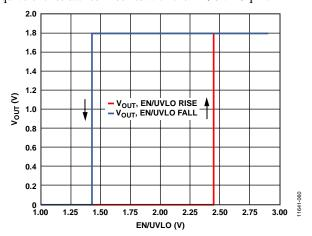
Figure 65. Typical VOUT Response to EN/UVLO Pin Operation
