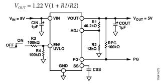
Figure 62. Typical Adjustable Output Voltage Application Schematic
