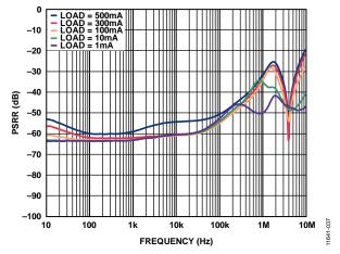
Figure 43. Power Supply Rejection Ratio vs. Frequency,  $V_{\rm OUT} = 5$  V,  $V_{\rm IN} = 6$  V, Adjustable
