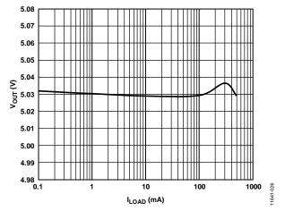
Figure 30. Output Voltage vs. Load Current,  $V_{OUT} = 5 V$ , Adjustable
