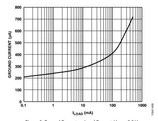
Figure 9. Ground Current vs. Load Current,  $V_{OUT} = 3.3 V$
