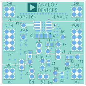
Figure 80. Example SOIC PCB Layout
