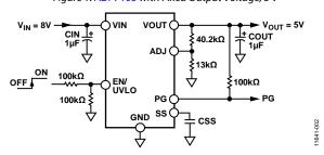
Figure 2. ADP7105 with Adjustable Output Voltage, 5 V
