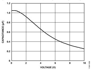
Figure 64. Capacitance vs. Voltage Bias Characteristic
