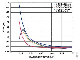
Figure 46. Power Supply Rejection Ratio vs. Headroom Voltage, 1 kHz,  $V_{\rm OUT}$  = 5 V
