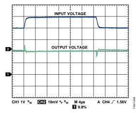
Figure 54. Line Transient Response,  $C_{IN}$  =  $C_{OUT}$  = 1  $\mu$ F,  $I_{LOAD}$  = 500 mA,  $V_{OUT}$  = 1.8 V
