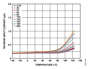
Figure 32. Reverse Input Current vs. Temperature,  $V_{IN} = 0 V$ , Different Voltages on  $V_{OUT}$
