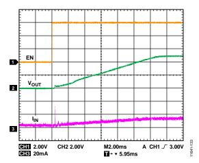
Figure 33. Start-Up Time,  $V_{EN}$  and  $V_{IN}$  = 6 V,  $C_{IN}$  and  $C_{OUT}$  = 1  $\mu$ F,  $C_{SS}$  = 10 nF,  $I_{OUT}$  = 10 mA,  $V_{OUT}$  = 5 V
