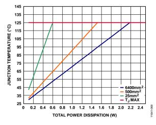
Figure 74. SOIC,  $T_A = 25$ °C
