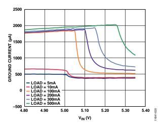
Figure 22. Ground Current vs. Input Voltage (in Dropout),  $V_{OUT} = 5 V$
