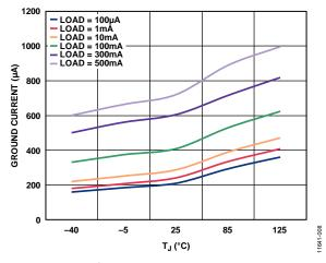
Figure 8. Ground Current vs. Junction Temperature,  $V_{OUT} = 3.3 \text{ V}$
