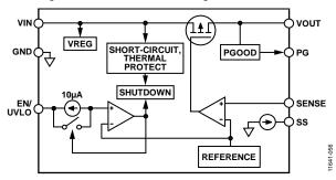
Figure 60. Fixed Output Voltage Internal Block Diagram
