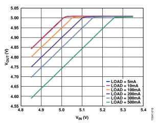
Figure 21. Output Voltage vs. Input Voltage (in Dropout),  $V_{OUT} = 5 V$
