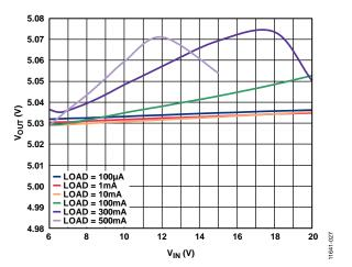
Figure 31. Output Voltage vs. Input Voltage,  $V_{OUT} = 5 V$ , Adjustable
