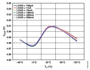
Figure 15. Output Voltage vs. Junction Temperature,  $V_{OUT} = 5 V$
