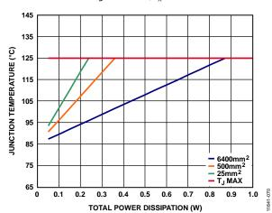
Figure 76. SOIC,  $T_A = 85$ °C
