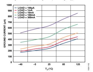
Figure 18. Ground Current vs. Junction Temperature,  $V_{OUT} = 5 V$
