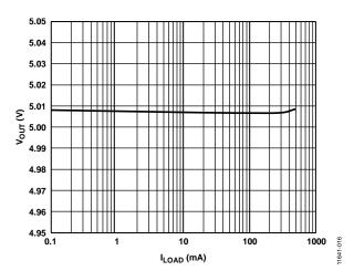
Figure 16. Output Voltage vs. Load Current,  $V_{OUT} = 5 V$
