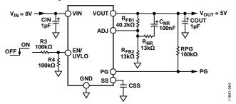
Figure 70. Noise Reduction Modification to Adjustable LDO Regulator
