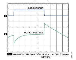
Figure 52. Load Transient Response,  $C_N = C_{OUT} = 1~\mu F$ ,  $I_{LOAD} = 1~mA$  to 500 mA,  $V_{OUT} = 3.3~V$ ,  $V_{IN} = 5~V$
