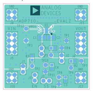
Figure 79. Example LFCSP PCB Layout
