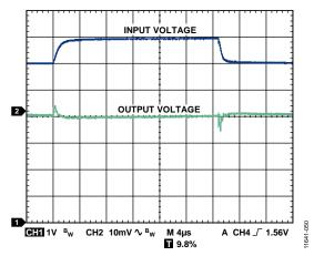
Figure 56. Line Transient Response,  $C_{IN}$  =  $C_{OUT}$  = 1  $\mu$ F,  $I_{LOAD}$  = 500 mA,  $V_{OUT}$  = 5 V
