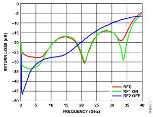
Figure 10. Return Loss vs. Frequency for RFC, RF1 On, and RF2 Off
