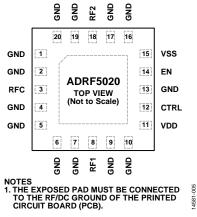
*Figure 5. Pin Configuration (Top View)*
