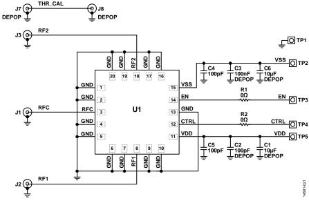
Figure 21. Evaluation Board Schematic
