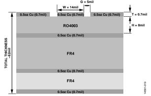
Figure 19. Evaluation Board (Cross Sectional View)
