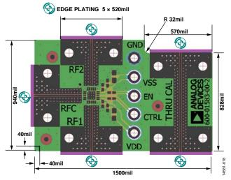
Figure 18. Evaluation Board Layout (Top View)
