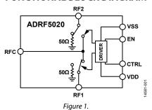
This broadband switch requires dual supply voltages, +3.3 V and -2.5 V, and provides CMOS/LVTTL logic-compatible control.
