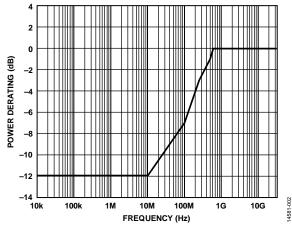
Figure 2. Power Derating for Through Path vs. Frequency, T<sub>CASE</sub> = 85°C
