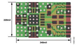
Figure 22. Probe Board Layout (Top View)
