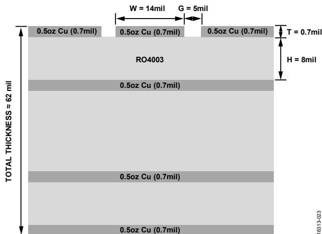
Figure 23. Evaluation Board (Cross Sectional View)
