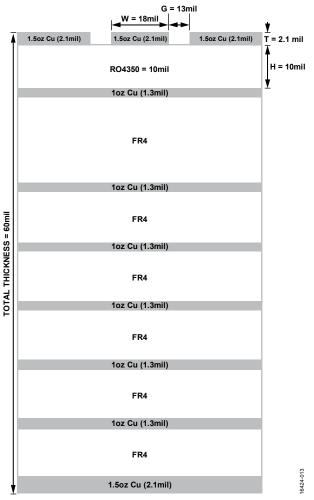
Figure 13. ADRF5132-EVALZ Evaluation Board Cross Sectional View
