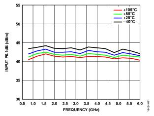
Figure 11. Input 0.1 dB Power Compression (P0.1dB) vs. Frequency over Temperature,  $V_{\rm DD} = 5~\rm V$
