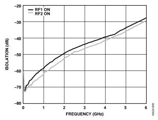
Figure 9. Isolation Between RF1 and RF2 vs. Frequency at  $V_{DD} = 5 V$ , Switch Mode On
