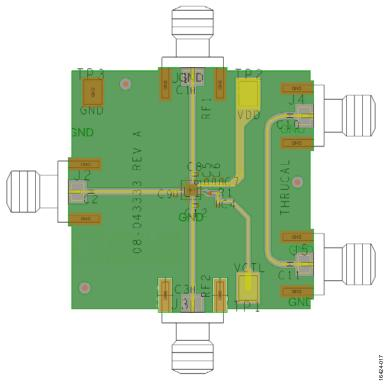
Figure 16. ADRF5132-EVALZ Evaluation Board Component Placement
