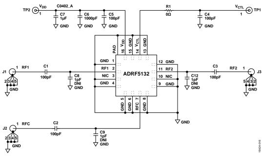
Figure 17. Application Circuit
