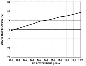
Figure 14. ADRF5132-EVALZ Evaluation Board Temperature Rise (Oven Temperature Set to 75°C)
