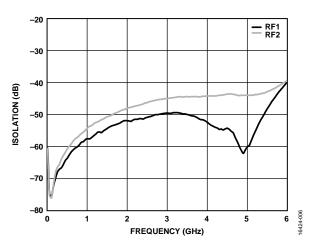
Figure 6. Isolation Between RFC and RF1/RF2 vs. Frequency at  $V_{\rm DD} = 5 \ V$
