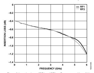
Figure 5. Insertion Loss of RF1 and RF2 vs. Frequency at  $V_{\rm DD} = 5 \ V$
