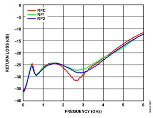
Figure 7. Return Loss vs. Frequency at  $V_{DD} = 5 V$
