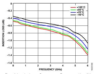
Figure 8. Insertion Loss vs. Frequency over Temperature,  $V_{DD} = 5 V$
