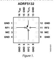
The on-chip circuitry operates at a single, positive supply voltage of 5 V and a typical supply current of 1.1 mA typical, making the ADRF5132 an ideal alternative to pin diode-based switches.
