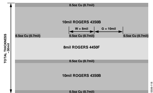
Figure 19. Evaluation Board Cross Sectional View
