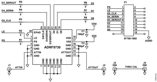
Figure 40. Evaluation Board Schematic
