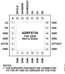
Figure 4. Pin Configuration
