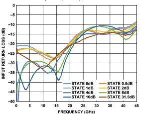
Figure 10. Input Return Loss vs. Frequency (Major States Only) with Impedance
