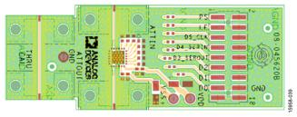
Figure 38. Evaluation Board, Top View
