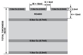
Figure 41. Probe Matrix Board Stackup
