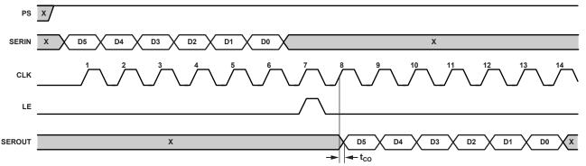
Figure 35. Serial Output Timing Diagram
