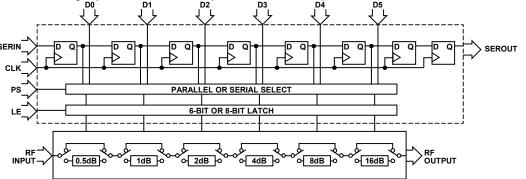
Figure 32. Simplified Circuit Diagram
