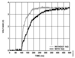
Figure 33. Using a Resistor on SEROUT
