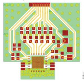
Figure 42. Probe Matrix Board Top View
