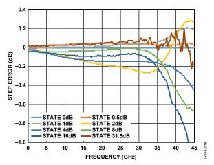
Figure 18. Step Error vs. Frequency (Major States Only) Without Impedance Match
