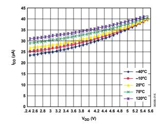
Figure 14. Operating Supply Current vs. Voltage Over Temperature
