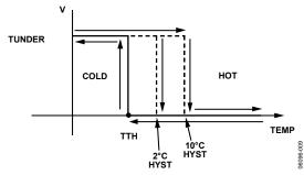
Figure 18. ADT6504 TUNDER Transfer Function
