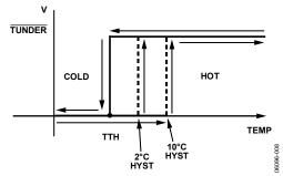
Figure 17. ADT6503 TUNDER Transfer Function
