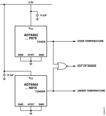
Figure 22. Temperature Window Alarms
