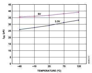
Figure 6. Operating Supply Current vs. Temperature
