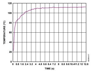
Figure 9. Thermal Step Response in Perfluorinated Fluid
