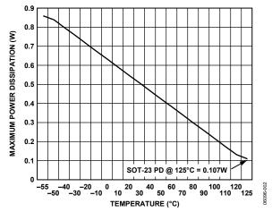
Figure 2. SOT-23 Maximum Power Dissipation vs. Temperature
