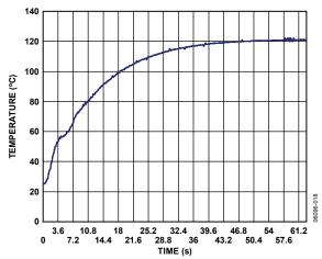
Figure 10. Thermal Step Response in Still Air
