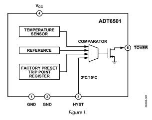
The ADT6503 and ADT6504 are used for monitoring temperatures from -45°C to +15°C only. Therefore, the logic output pin becomes active when the temperature goes lower than the selected trip point temperature.
