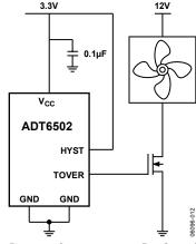
Figure 21. Overtemperature Fan Control
