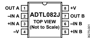
Figure 1. 8-Lead SOIC_N (R-8)
