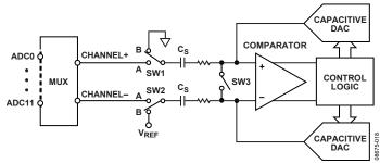
Figure 25. ADC Conversion Phase
