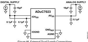
Figure 46. External Dual Supply Connections
