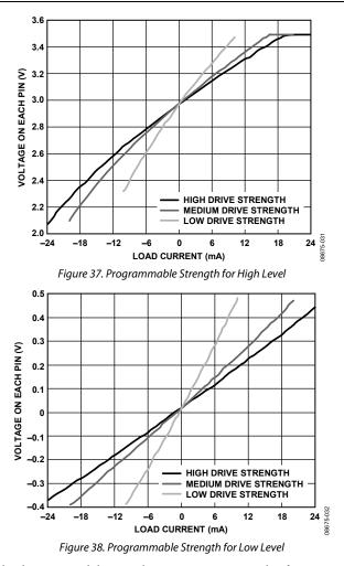
The drive strength bits can be written one time only after reset. More writing to related bits has no effect on changing drive strength. The GPIO drive strength and pull-up disable is not always adjustable for the GPIO port. Some control bits cannot be changed (see Table 59).
