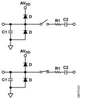
Figure 27. Equivalent Analog Input Circuit Conversion Phase: Switches Open, Track Phase: Switches Closed
