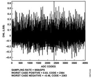
Figure 10. Typical DNL,  $f_{ADC} = 950$  kSPS, Internal Reference Used
