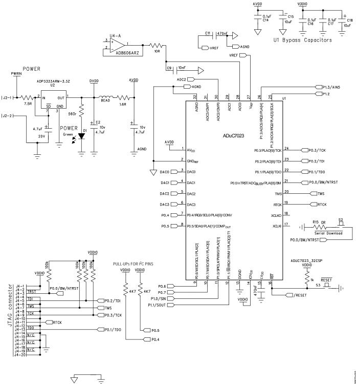
Figure 54. Typical System Configuration
