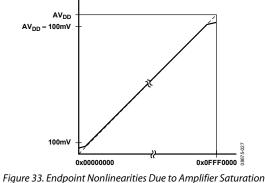
Figure 55. Enapoint Nonlineanties Due to Ampliner Saturation
