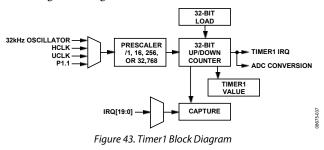
The Timer1 interface consists of five MMRs: T1LD, T1VAL, T1CON, T1CLRI, and T1CAP.
