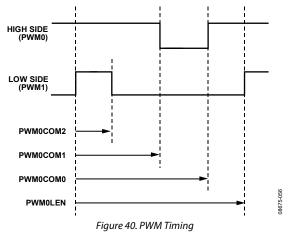
The PWM clock is selectable via PWMCON1 with one of the following values: UCLK divided by 2, 4, 8, 16, 32, 64, 128, or 256. The length of a PWM period is defined by PWMxLEN.
