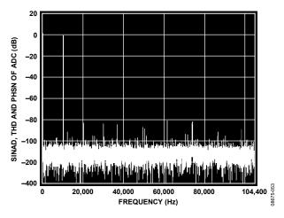
Figure 14. SINAD, THD, and PHSN of ADC, Internal 2.5 V Reference Used
