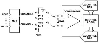
Figure 24. ADC Acquisition Phase
