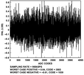
Figure 12. Typical DNL, f<sub>ADC</sub> = 950 kSPS, External 1.0 V Reference Used
