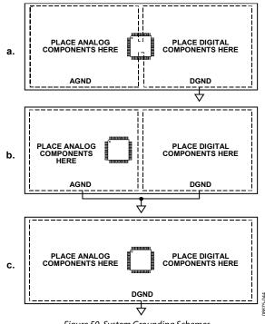
Figure 50. System Grounding Schemes
