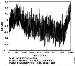
Figure 11. Typical INL, f<sub>ADC</sub> = 950 kSPS, Internal Reference Used
