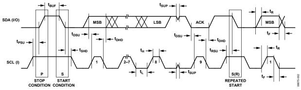
Figure 2. I<sup>2</sup>C-Compatible Interface Timing
