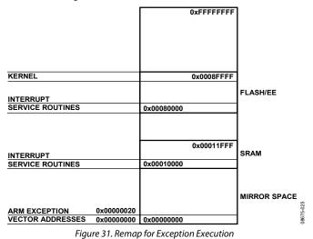
By default, and after any reset, the Flash/EE is mirrored at the bottom of the memory array. The remap function allows the programmer to mirror the SRAM at the bottom of the memory array, which facilitates execution of exception routines from SRAM instead of from Flash/EE. This means exceptions are executed twice as fast, being executed in 32-bit ARM mode with 32-bit wide SRAM instead of 16-bit wide Flash/EE memory.
