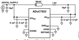
Figure 47. External Single Supply Connections
