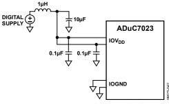
Figure 48. Recommended IOV<sub>DD</sub> Supply Filter
