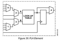
In total, 20 GPIO pins are available on the ADuC7023 for the PLA. These include 11 input pins and nine output pins, which need to be configured in the GPxCON register as PLA pins before using the PLA.
