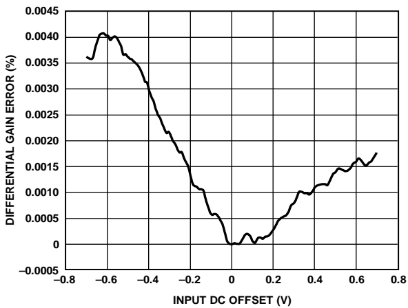
Figure 45. ADV3228 Differential Gain Error
