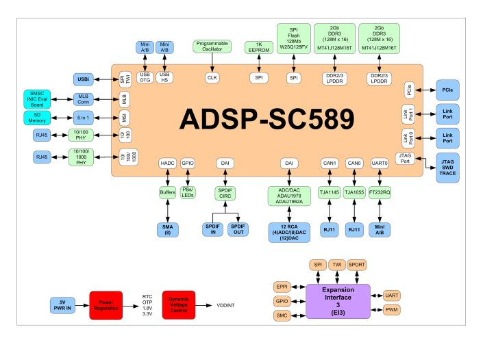
The ADSP-SC589 EZ-Board has two 25 MHz input clocks and runs at a max core clock frequency of 450 MHz. The input clock frequency can be changed through the SI5356A I2C programmable clock generator.
