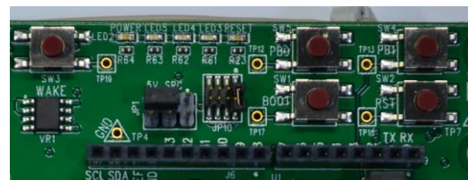
Figure 4. EZ-Kit Push Buttons Located Near the LEDs
