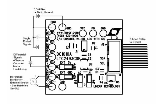
Figure 1. Proper Measurement Equipment Setup
