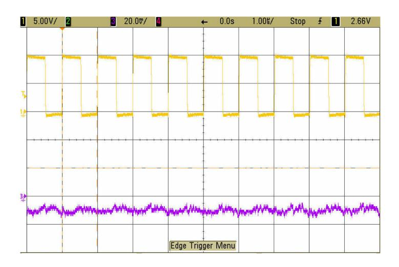
Figure 3. Switch Waveform & Output Ripple Voltage  $V_{IN} = 8.4V, \ V_{OUT} = 3.3V, \ I_{OUT} = 2.5A, \ Fsw = 1 \ MHz$ Trace 1: Switch Voltage (5 V/div)
