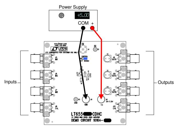
Figure 1. Recommended Demo Circuit Setup
