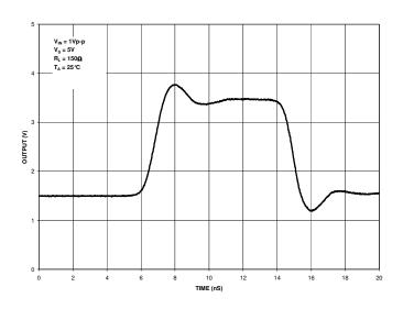
Figure 3. Typical Time-Domain Transmission Response
