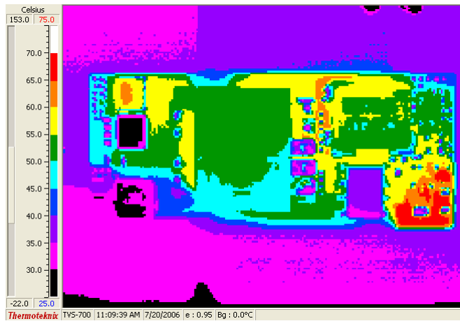
Figure 10. Temp Data (72Vin, 20A, 25°C, 200LFM airflow – front)
