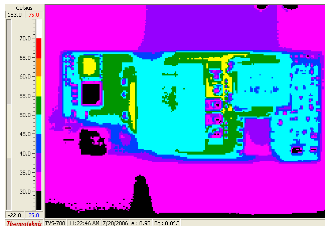
Figure 8. Temp Data (36Vin, 20A, 25°C, 200LFM airflow – front)
