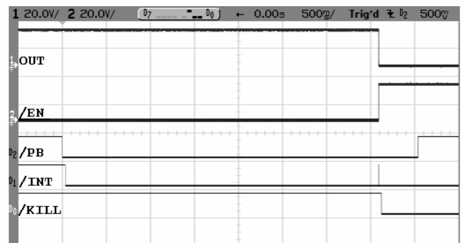
(b) Push Button Turn Off (PDT = 0.47uF, 500ms/div)
