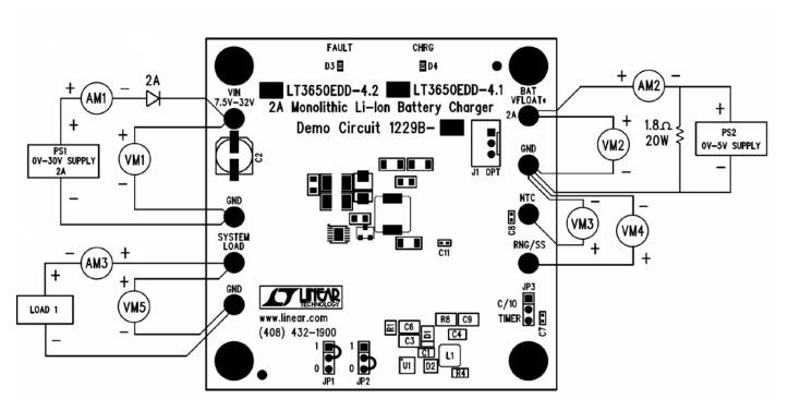
**Note:** Put a blocking diode between the input supply and the  $V_{\text{IN}}$  terminal. Kelvin connect the voltage meters directly to the board terminals as shown on the diagram. Use twisted pair input and output leads.
