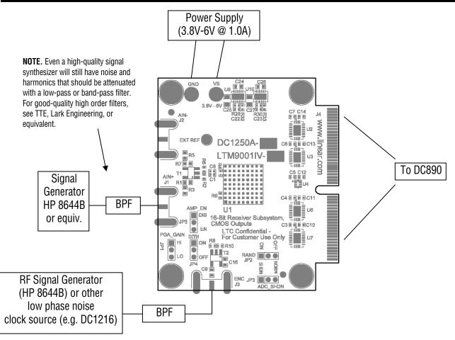
Figure 1. Proper Evaluation Equipment Setup
