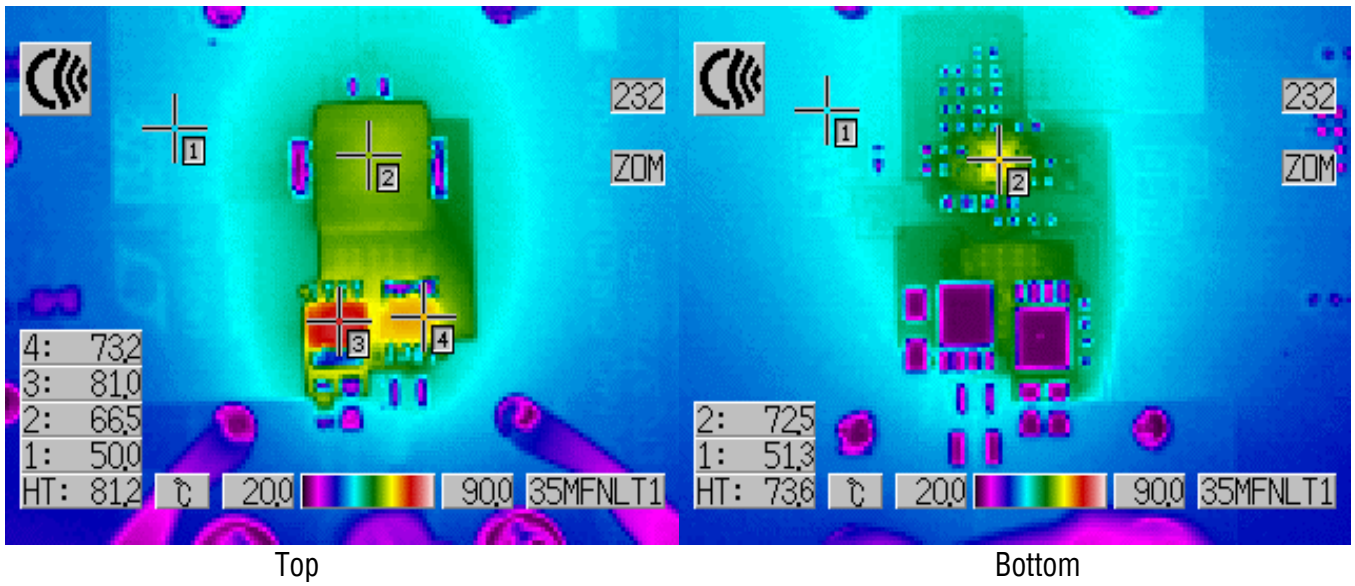
Figure 5. Thermal images of DC1290A-A, 26V IN , 1.2V OUT @ 15A, 22°C ambient
