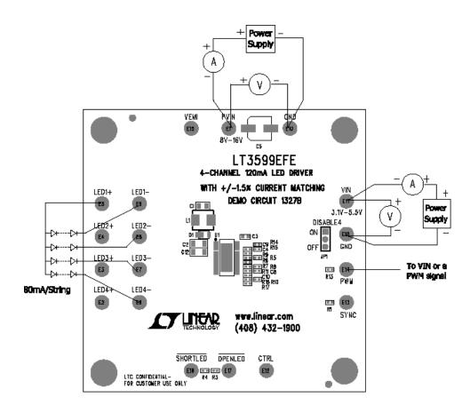
Figure 1. Proper Measurement Equipment Setup
