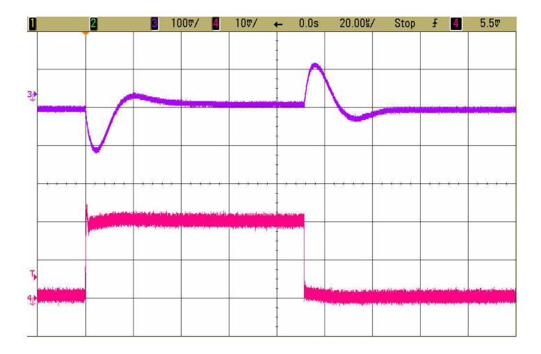
Figure 4. Load Step Response V<sub>IN</sub> = 3.3V, V<sub>OUT</sub> = 1.8V, 4A Load Step (0.1A <-> 4A) Forced Continuous Mode Fsw = 2 MHz External Compensation: Rith = 12.7k, Cith = 220 pF Trace 3: Output Voltage (100mV/div AC) Trace 4: Output Current (2A/div)
