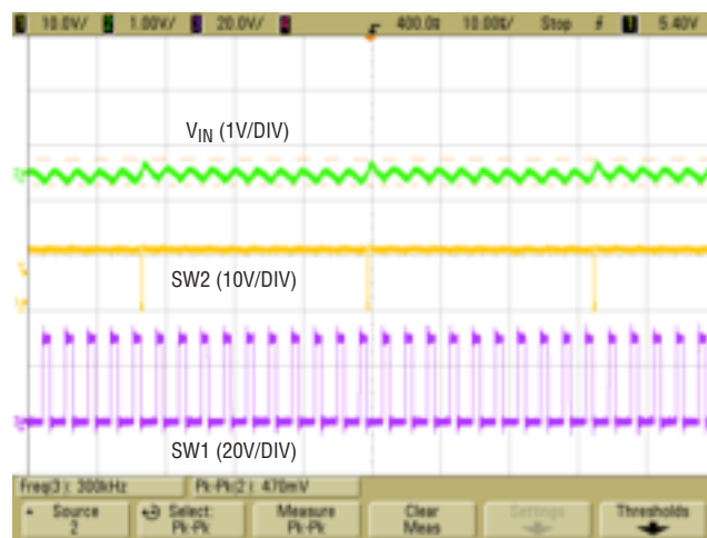
V_{IN} = 10V , V_{OUT} = 30V , I_{OUT} = 3A W/ INPUT FILTER: STUFF L2, L3, AND C_{IN2} V_{IN} PEAK-TO-PEAK RIPPLE = 0.47V
