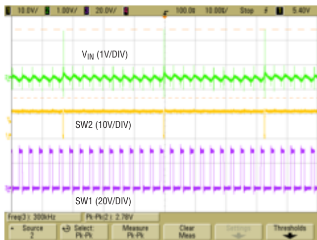
V_{IN} = 10V , V_{OUT} = 30V , I_{OUT} = 3A W/O INPUT FILTER: SHORT L2 AND L3. REMOVE C_{IN2} V_{IN} = PEAK-TO-PEAK RIPPLE = 2.78V
