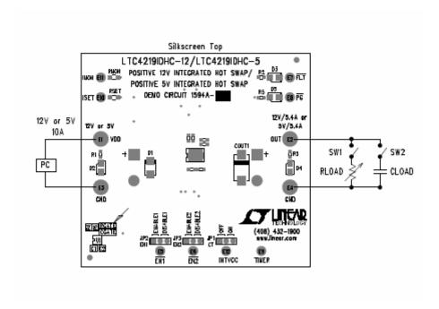
Figure 1. Proper Equipment Measurement Set-Up
