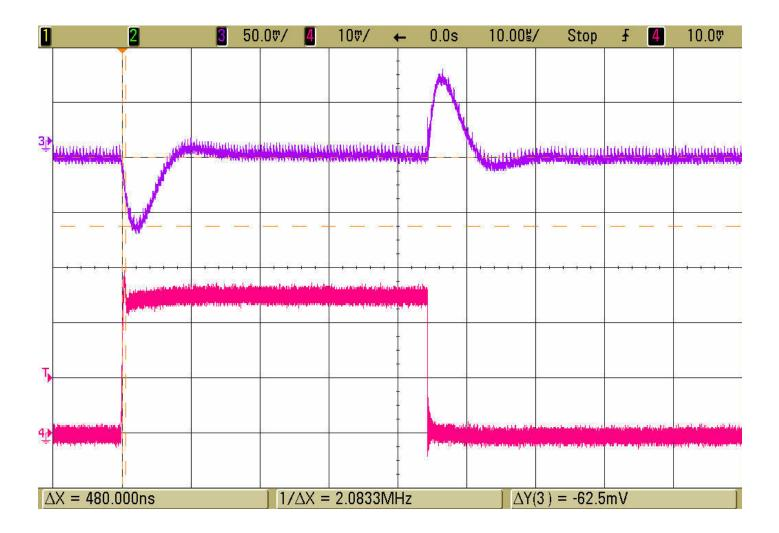
Figure 4. Load Step Response  $V_{IN} = 12V, V_{OUT} = 1.8V, 2.5A$  Load Step (OA <-> 2.5A) Forced Continuous Mode Fsw = 2 MHz
