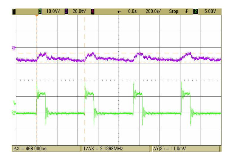
Figure 3. Switch Node & Output Ripple Voltage Waveforms  $V_{IN} = 12V$ ,  $V_{OUT} = 1.8V$ ,  $I_{OUT} = 2.5A$ ,  $F_{SW} = 2$  MHz Trace 3: Output Ripple Voltage (20 mV/div AC) Trace 2: Switch Voltage (10 V/div)
