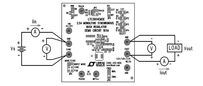
Figure 1. Proper Equipment Measurement Set-Up
