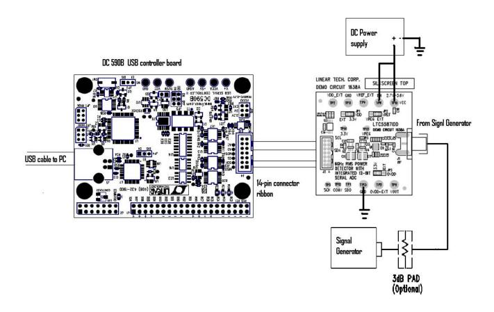
Figure 2. Proper test setup to connect DC1638A demo board to DC590A
