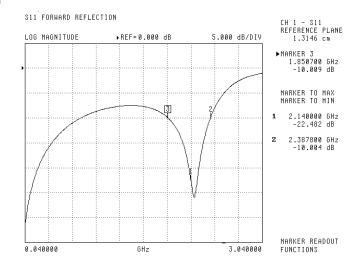
Figure 1. Standard Demo Board Return Loss
