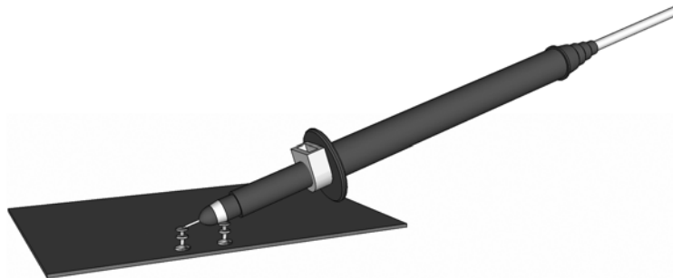
Figure 2. Measuring Input or Output Ripple
