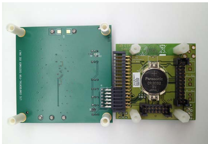
Figure 6. DC1923A Connected to DC9003A Dust Mote (Bottom View)
