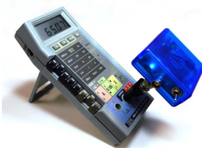
Figure 5. Completed Unit Attached to DMM
