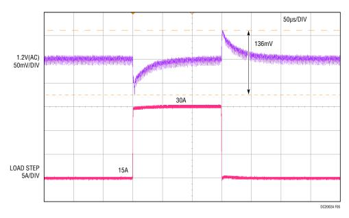
Figure 5. 50% to 100% to 50% Load Step Response of the 1.2V Rail.  $C_{OUT}$  = 3× Sanyo 2R5TPE330M9 || 2× 100 $\mu$ F X5R 1206, L = Würth 744301033 (0.33 $\mu$ H), f<sub>SW</sub> = 400kHz.
