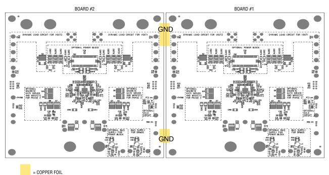
Figure 6. How to Parallel Two Boards for a Single Output, 4 Phase Converter
