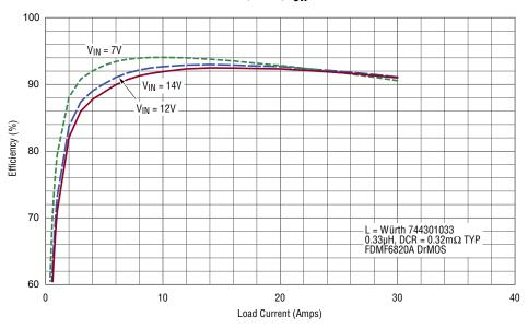
Figure 2. Efficiency Curves for the 1.5V Rail at  $V_{\text{IN}}$  = 12V, 14V and 7V in CCM.
