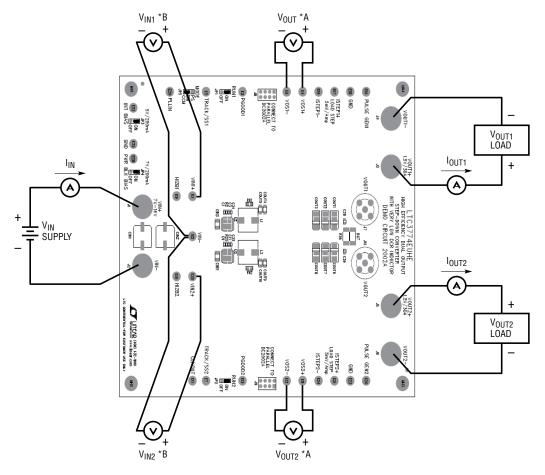
\*A MONITOR THE OUTPUT VOLTAGE ACROSS EITHER COUT4 OR COUT9 FOR ACCURATE EFFICIENCY MEASUREMENTS. \*B MONITOR THE VOLTAGE AT VIN1 WHEN MEASURING THE EFFICIENCY OF PHASE 1 AND VIN2 WHEN MEASURING THE EFFICIENCY OF PHASE 2.
