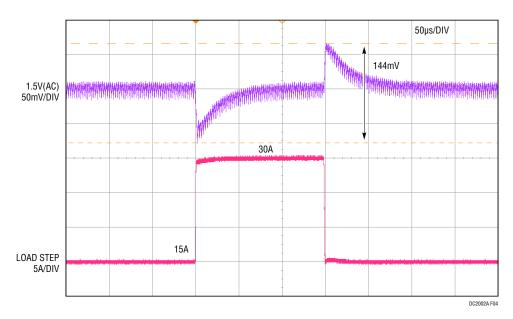
Figure 4. 50% to 100% to 50% Load Step Response of the 1.5V Rail.  $C_{OUT}$  = 3× Sanyo 2R5TPE330M9 || 2× 100 $\mu$ F X5R 1206, L = Würth 744301033 (0.33 $\mu$ H), f<sub>SW</sub> = 400kHz.
