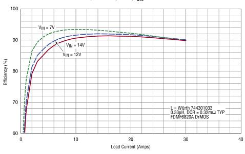
Figure 3. Efficiency Curves for the 1.2V Rail at  $V_{\text{IN}}$  = 12V, 14V and 7V in CCM.
