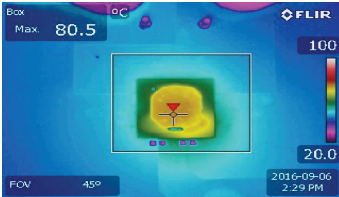
Figure 4. Thermal Image of LTM4636, V_{IN} = 12V , V_{OUT} = 1.0V , I_{LOAD} = 40A , Ambient Temperature = 23.0^{\circ}C , No Forced Airflow
