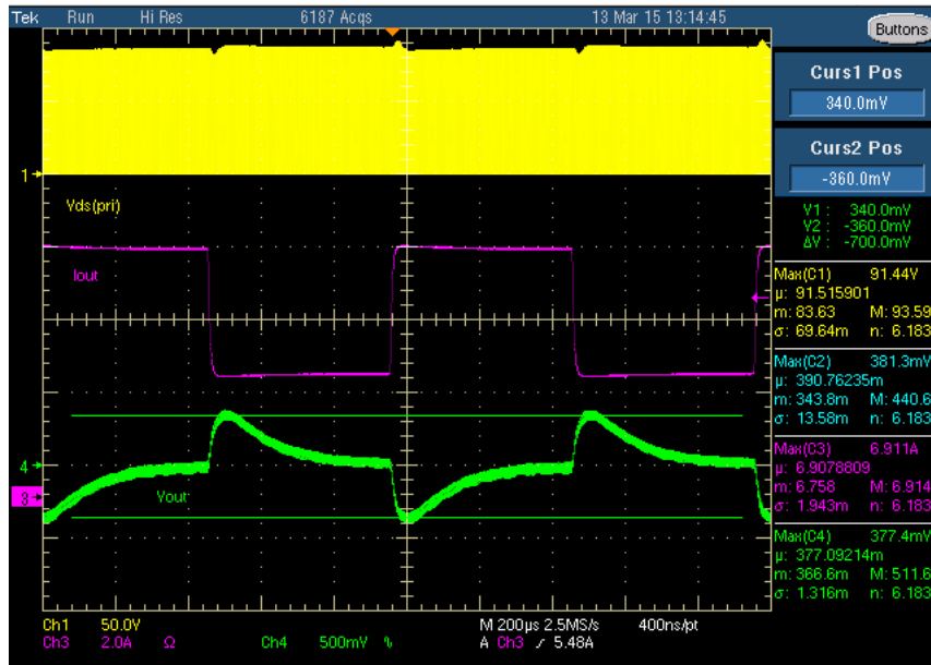
Figure 6. Load Transient Response ( V_{PORT} = 57V , 3.5A to 7A to 3.5A)
