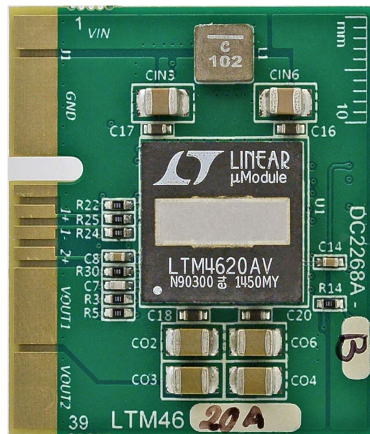
Figure 1. LTM4620A/DC2268A-B Demo Board
