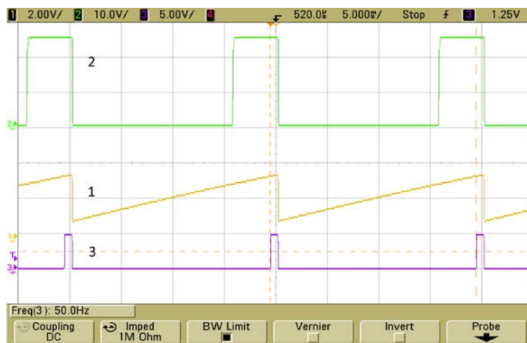
Figure 3. Short-Circuit with Automatic Restart Voltage Waveforms. CH 1 Pin 2 (TIMER), CH 2 VOUT, CH 3 Pin 3 (FAULT).
