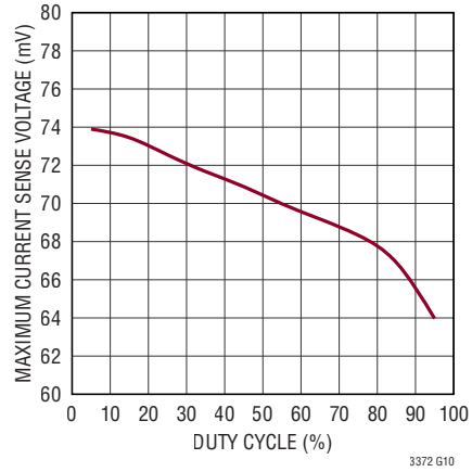
Maximum Current Sense Threshold vs Duty Cycle
