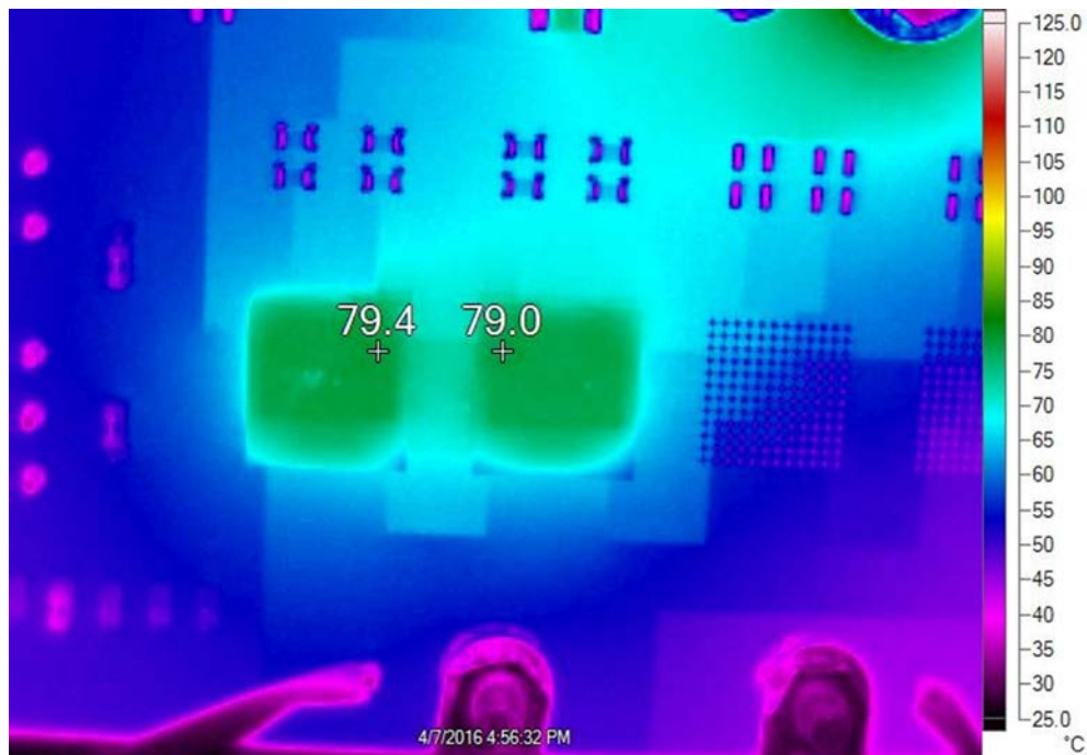
Figure 6. Thermal Performance at V_{IN} = 12V , V_{OUT} = 1V , I_{OUT} = 100A , T_A = 23.8^\circ C , 200LFM Air Flow
