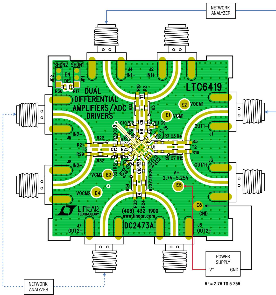
Figure 1. Proper Equipment Setup for Frequency Response Measurement
